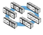
Doors can slide at any unoccupied position. By adding more doors, the more opening patterns will be possible.
