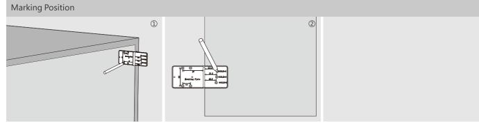
① Mark the position of the mounting plate screw holes
