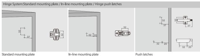
Standard mounting plate In-line mounting plate
