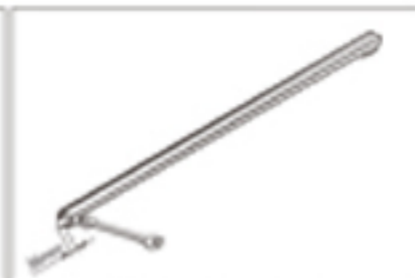
Fix the lower stopper with 5mm spanner
