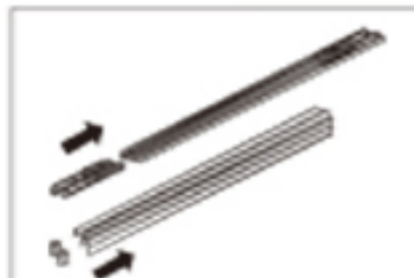
Insert the damper into top track Insert the lower stopper into bottom track
