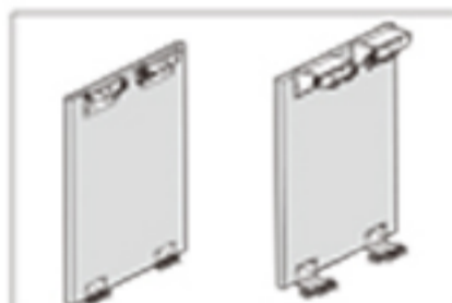
Install inner door top and out door's top and bottom roller
