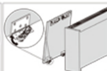
Open the anti-drop device on bottom roller before mounting the inner door
