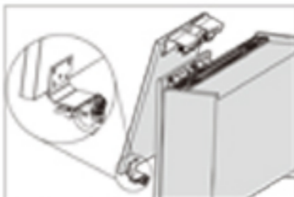
Open the anti-drop device on bottom roller before mounting the outer door
