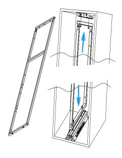
3.Insert fitting A into the big hole on frame as following.
