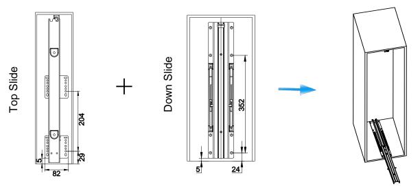
2.Insert the frame into slide, adjust the short support to combine with top slide, then screw on it.
