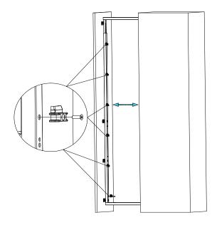
4.Insert bracket to door panel with fitting A, the screws can be adjusted to match with cabinet door.
