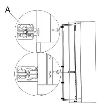
5.Install fitting on the inside of the support frame according to the installation method shown below. Height can be adjusted for personal use.
