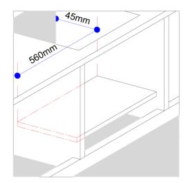
The panels of the adjacent cabinets must be made of heat resistant material. In particular, cabinets with a veneer exterior must be assembled with glues which can withstand temperature of up to  $100^{\circ}$ C
