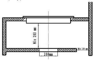
**IMPORTANT:** when installing the appliance above a cupboard, a dividing shelf, as shown above, must be installed.
