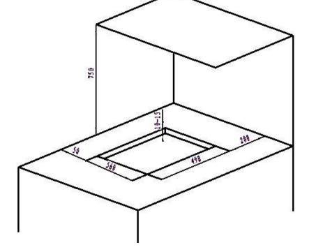
Create an opening with the dimensions shown in the paragraph 10.1 in the top surface of the counter, keeping a minimum distance of 50mm from the rear edge.
