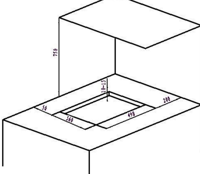
Create an opening with the dimensions shown in the paragraph 10.1 in the top surface of the counter, keeping a minimum distance of 50mm from the rear edge.
