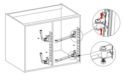
To adjust the position of the curve arm and straight bar
