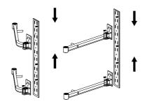
3. Mounting of gas spring and buffer
